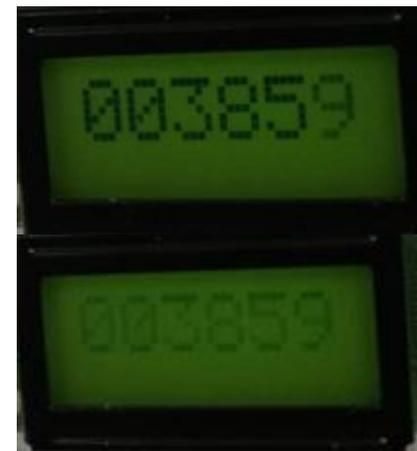
At the end of the sequence all 6 digits will flash, during this time press and hold the button for 3 seconds and release and the display should say DONE. Power the gauge off and then on again and the saved mileage should be displayed.
