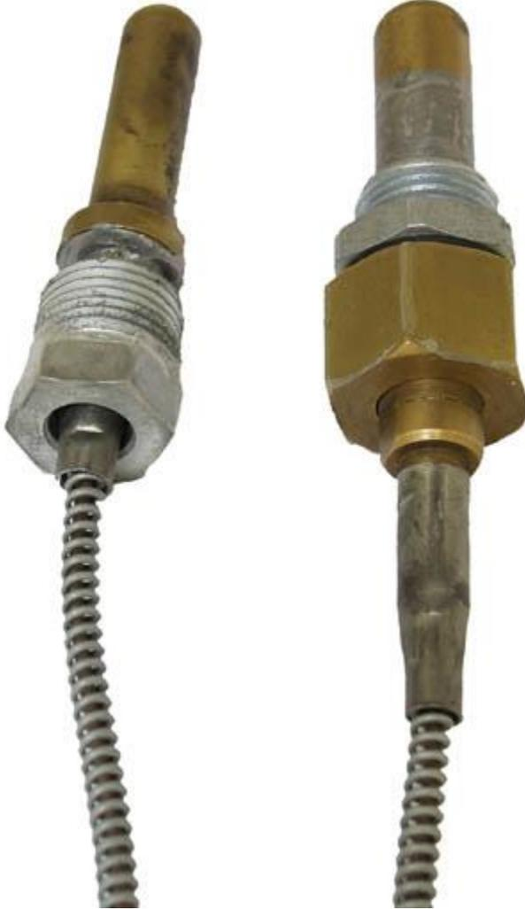
Dual gauges with a temperature scale have an ether filled bulb fitted at the end of the armoured capillary tubing.
